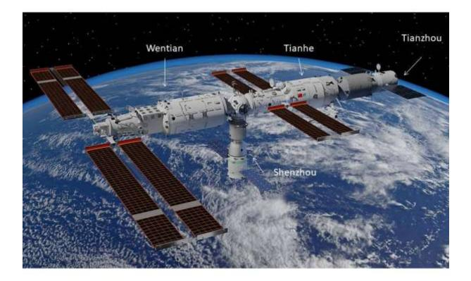
Rendering of the Tiangong Space Station in its current construction state as of August 2022: the *Tianhe* core module with docking node (launched April 29, 2021 on a CZ-5B) in the middle, *Wentian* second core module (launched July 24, 2022 on a CZ-5B) on the left, *Tianzhou-4*, robotic cargo craft, (docked May 9, 2022, launched with a CZ-7) on the right and the Shenzhou crew vehicle docked at the nadir of the multiple port docking node. (image by Shujianyang - Own work, CC BY-SA 4.0). [7]
